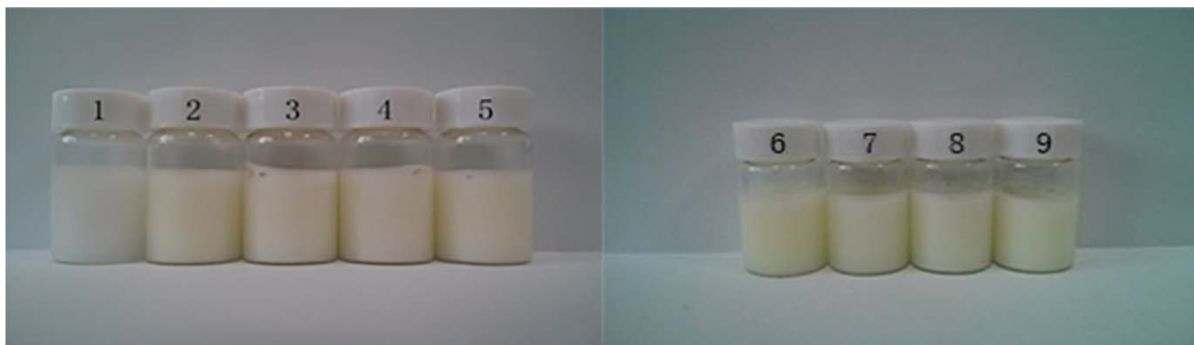
Figure 14. The emulsion stability of aqueous “two-phase” polymerization of AM in PEG aqueous solution mediated by CTA after 1 month standing at ambient temperature. The number corresponds to the reaction numbers in Table I. [Color figure can be viewed in the online issue, which is available at wileyonlinelibrary.com .]
